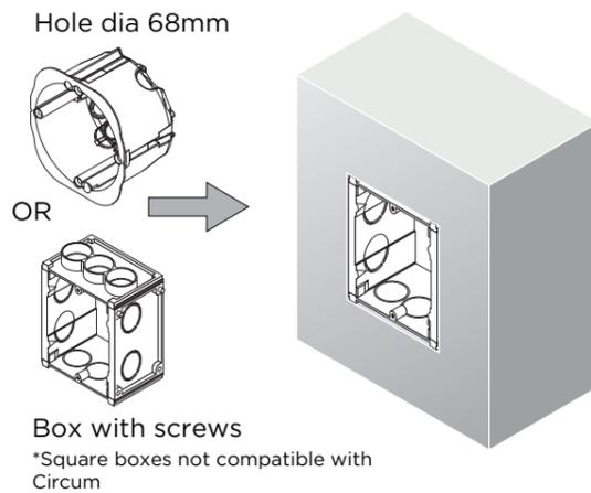
**2 FIX FRAME TO WALL OR JUNCTION BOX WITH 2 SCREWS (USE HOLES ON VERTICAL AXIS)**
