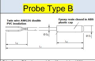
D1 = 9 mm D2 = 4 mm L2 = 49 mm L1 = 1250 mm
