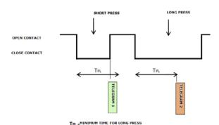
When contact is closed and the debounce time is over then counting time to contact closure starts; if the contact is opened again (note that debounce time is considered also in contact opening) before time exceeds TPL time, device executes the command associated with the event of "short press" and if, on the contrary, TPL timeout expires and contact is still closed then the command associated with the event of "long press" is executed.
