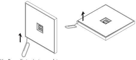
\*Use Paperclip to eject coverplate
